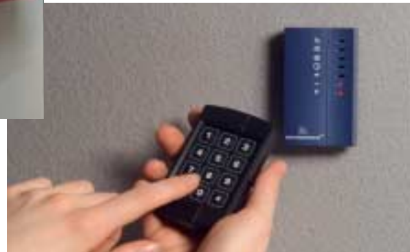
Removing of lost tags using remote programmer
